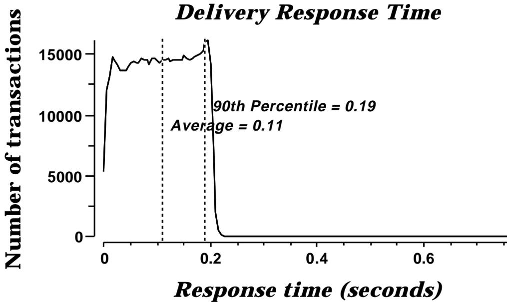
Figure 6-3-5. BULL ESCALA EPC2450 Delivery (Deferred) Response Time Distribution
