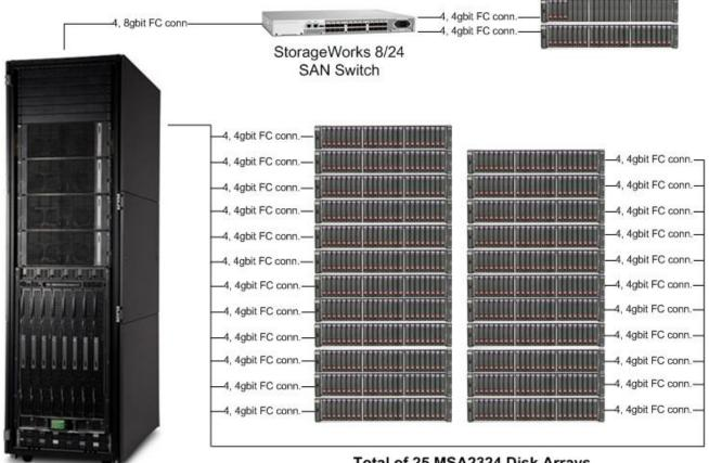
HP Integrity SuperDome 2 Itanium/1.73 GHz/24 MB iL3/16p/64c
