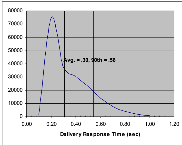
Figure 5-4. Delivery Transaction - Response Time Frequency Distribution
