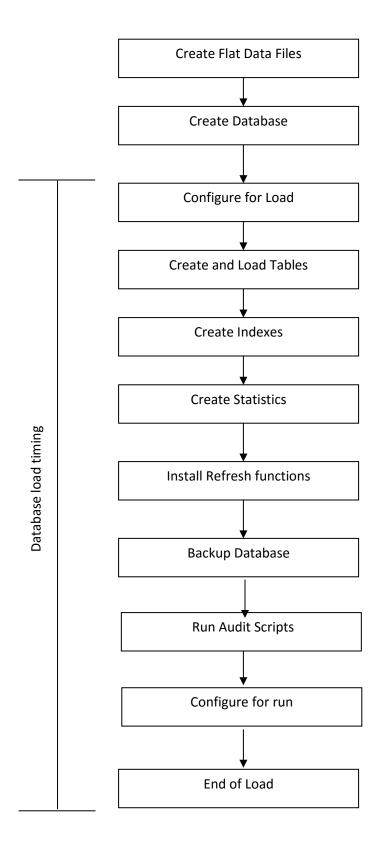
Figure 4.8: Block Diagram of Database Load Process
