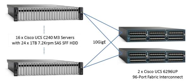
The measured configuration consisted of:
