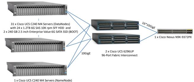
with with 24 x 1.2TB 6G SAS 10K rpm SFF HDD 2 x 240 GB 2.5 inch Enterprise Value 6G SATA SSD (BOOT)
