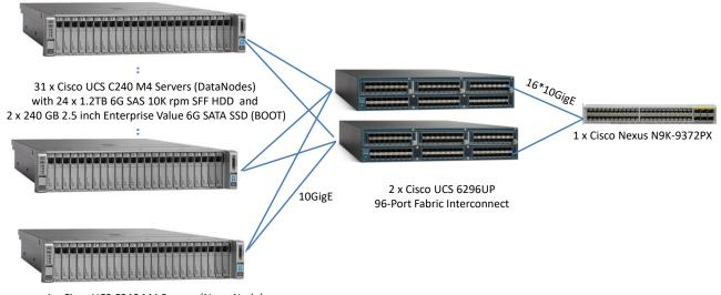
1 x Cisco UCS C240 M4 Servers (NameNode) with with 24 x 1.2TB 6G SAS 10K rpm SFF HDD 2 x 240 GB 2.5 inch Enterprise Value 6G SATA SSD (BOOT)
