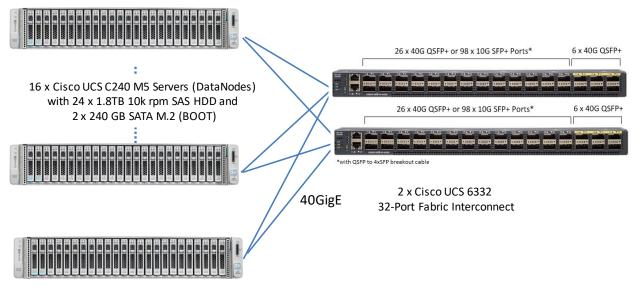
1 x Cisco UCS C240 M5 Server (NameNode) with 2 x 1.8TB 10k rpm SAS HDD and 2 x 240 GB SATA M.2 (BOOT)
