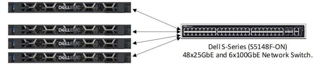
3x Dell PowerEdge R6415 Servers (Data Nodes) 1x AMD EPYC 7401P 24-Core Processor 256 GB (8x 32GB RDIMM 2666MT/s Dual Rank) 1x 120GB SSD SATA 2.5in Hot-plug Drive 1x 1.6 TB Dell NVMe 1x Mellanox Dual Port 25GbE SFP28 NIC
