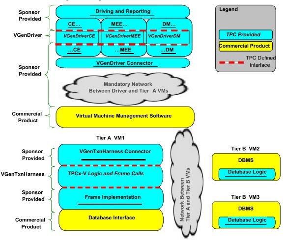
Figure 10.c - Functional Components of the Test Configuration
