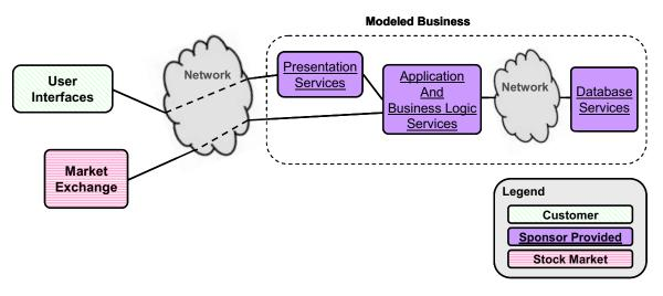
Figure 10.b - Abstraction of the Functional Components in an OLTP Environment
