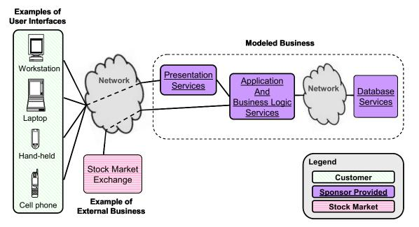
Figure 10.a - Diagram of the Real-World OLTP Environment
