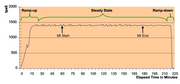
Figure 5c - Example of the Measured Throughput versus Elapsed Time Graph
