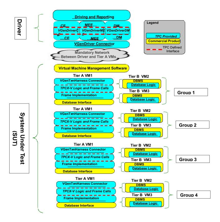
Figure 10.d - Defined Components of the Test Configuration
