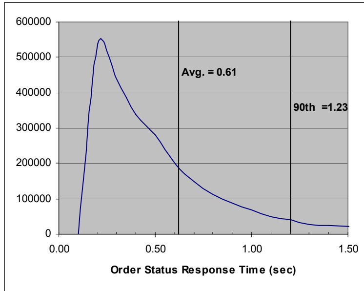
Figure 5-4. Delivery Transaction - Response Time Frequency Distribution
