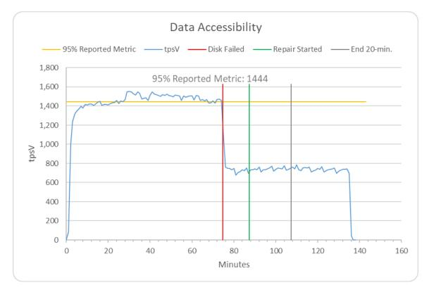
Figure 7-1 Data Accessibility Test Run Graph
