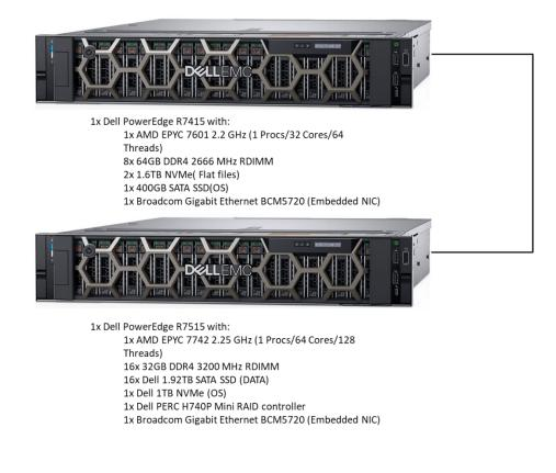
Figure 1-1 Measured Configuration
