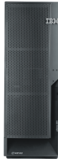
1 x IBM xSeries 225 1 x 2.4GHz/512MB Xeon Processor 3 x Mylex AcceleRAID A352 Adapters 1 x 18.2GB Drive 2 x 73.4GB Drives
